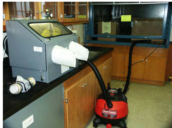
Figure 1: “Fully enclosed” blasting cabinet with gloved portals. Interior workspace dimensions are approximately 0.6 m wide x 0.4 m deep x 0.4 m high.
