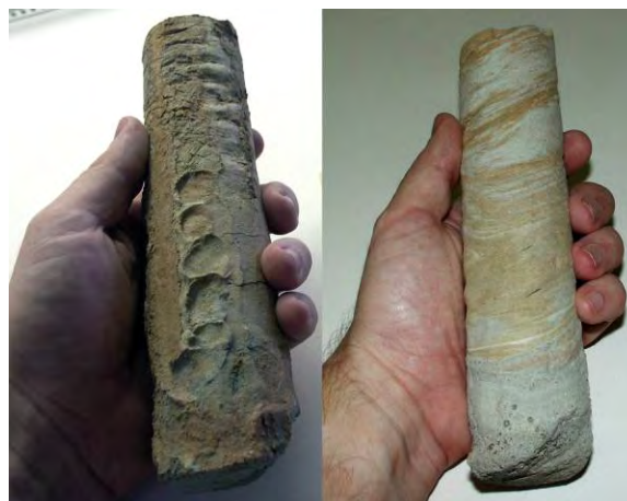
Figure 2: Before and after images of core cleaned by abrasive (sand) blasting. Note the colors and structures not visible before blasting. In spite of the core being poorly lithified, little material has been artificially eroded by the abrasive blasting process.
