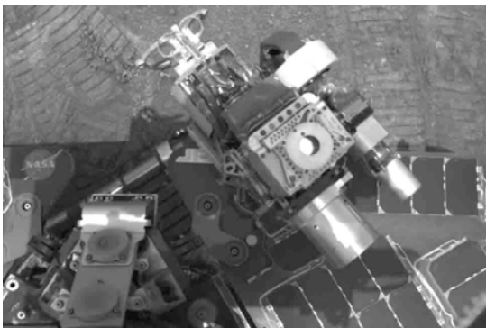
Figure 1: View from the pancam of the MI placed on the Spirit solar array on sol 505.
