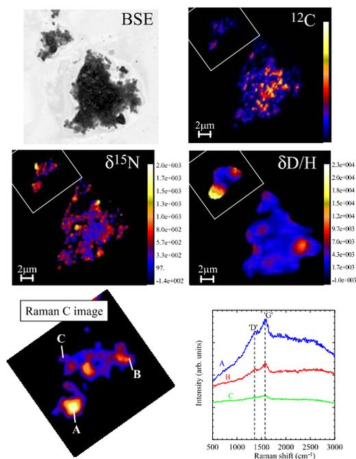
**Figure 1:** Back-scattered-electron, isotopic and Raman images of IDP L2054 E1. Bottom right shows three Raman spectra for two D hotspots (A and B) and a  $^{15}\text{N}$  hotspot (C). Area of Raman image is indicated on isotopic images.
