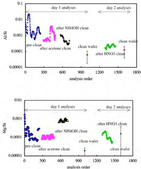
**Fig. 1** Step washing effects on Wafer 60045. Pre-clean, after acetone clean and after  $\text{NH}_4\text{OH}$  clean were analyzed on the same day, and the average of 6 analyses, with +3 sigma, on a clean control Si wafer is plotted at 1000 s for comparison. After  $\text{HNO}_3$  clean was analyzed on a second day, and the average of 11 analyses, with +3 sigma, on a clean control Si wafer is plotted at 1600 s for comparison.
