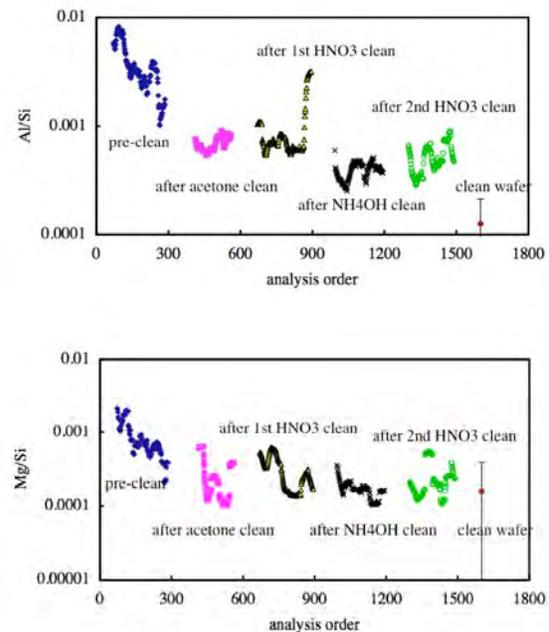
**Fig. 2** Step washing effects on Wafer 60044. The average of 11 analyses, with +3 sigma, on a clean control Si wafer is plotted at 1600 s for comparison.
