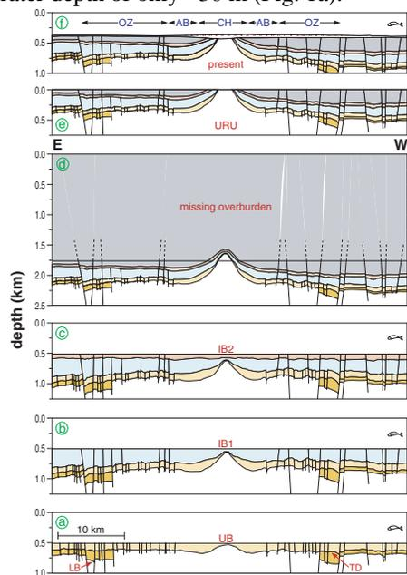
**Fig. 1.** Reconstruction of the Mjølnir original crater relief along an E-W trending profile by decompaction and fault restoration of the entire post-impact sedimentary succession. Time steps (a-f) correspond to the main unit boundaries. CH, central high; AB, annular basin; OZ, outer zone (modified from [3]).
