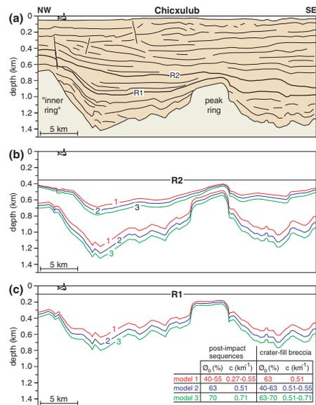
**Fig. 2.** Reconstruction of the Chicxulub original crater along (a) a re-interpreted depth-converted profile (part of profile Chicx-B [5]) by backstripping and decompaction utilizing paleowater depths of 350 m and 100 m for time-steps at reflectors R2 (b) and R1 (c), respectively.
