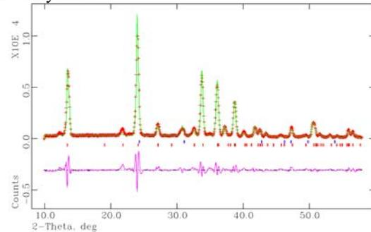
Figure 3. Rietveld refinement results for gypsum sample (97% gypsum-red vertical lines, 3% quartz-blue vertical lines).
