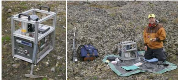
Figure 1. CheMin instrument in the Arctic
