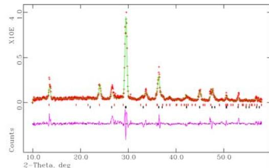
Figure 4. Refinement results for chicken-wire anhydrite sample (74% anhydrite, 26% gypsum).
