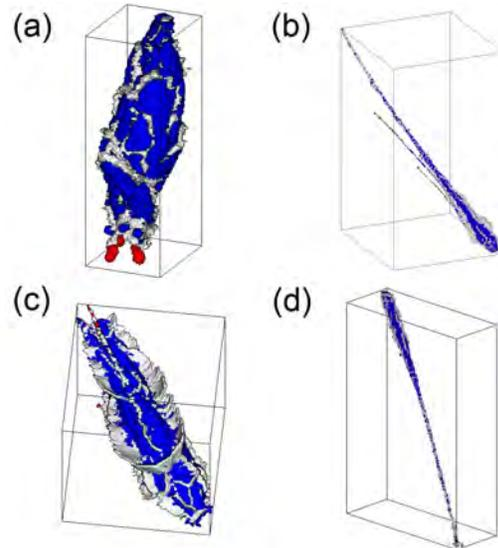
Figure 2. External shapes of impact tracks. (a) Track 67 namekuji (113  $\mu\text{m}$ ). (b) Track 68 skyrocket (2484  $\mu\text{m}$ ). (c) A bulbous portion near the entrance of (b). (d) Track 47 gobou (884  $\mu\text{m}$ ). Gray: track cavity. Blue: condensed aerogel. Red: captured particle.
