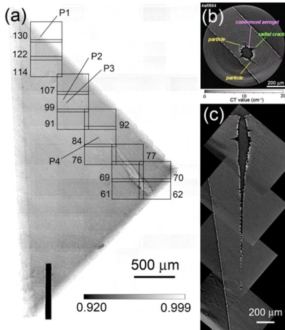
Figure 1. C2126,2,68,0 (skyrocket). (a) Tilted radiograph. Areas for XRF analyses are shown by boxes ( $400 \times 260 \mu\text{m}^2$ ). Four particles (P1-P4) were also analyzed by smaller areas ( $40 \times 40 \mu\text{m}^2$ ). A gray scale shows an x-ray transmittance. (b) A CT slice. (c) A CT image cut nearly parallel to the track.
