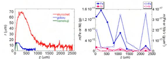
Figure 3. Track shapes and elemental distribution. (a) Mean track radius,  $r$ , vs. distance from the entrance,  $z$ . (b) Distribution of Fe and Ni along track 68 skyrocket.
