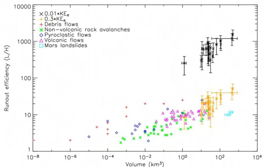
**Fig 2:** Runout efficiency ( $L/H$ ) versus flow volume. Martian fluidized ejecta and landslides, and a few terrestrial mass movements. Terrestrial data from [3, 4]
