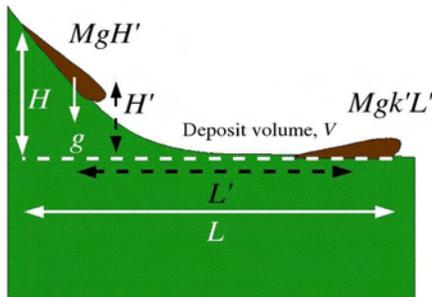
**Fig. 1:** Schematic illustrating how runout efficiency is measured at terrestrial landslides.
