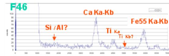
Figure 4. Example of the XRF spectrum acquired for a basaltic rock.
