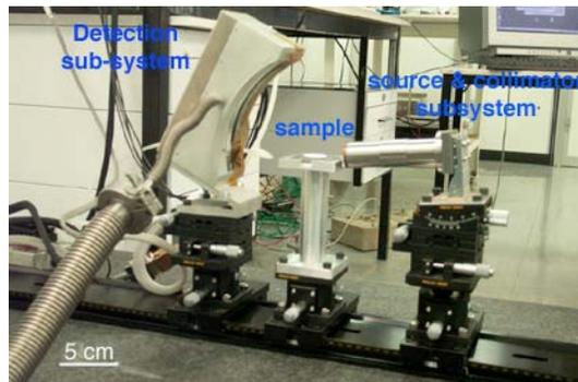
Figure 2. MARS-XRD breadboard.
