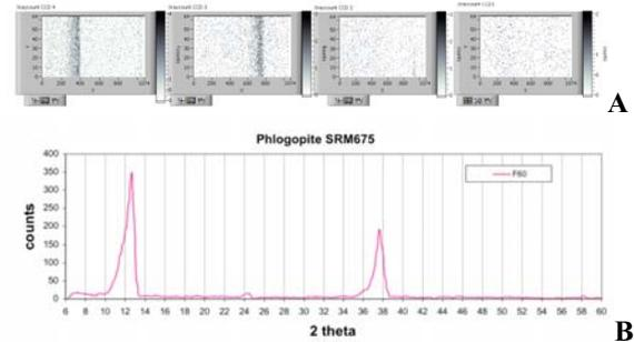
Figure 3. The diffraction pattern of Phlogopite (Phyllosilicates Family, NIST standard SRM675 acquired with the prototype). A. Windows of the GSE software showing each CCD image during acquisition of the diffraction pattern. B: Derived diffractogram at  $^{55}\text{Fe}$  wavelength (2.1 Angstrom).
