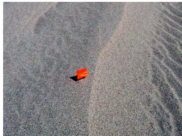
Figure 2. Oblique view of granule ripple showing 10.5 cm movement (to right) in 1380 minutes since flag was inserted on crest. Flag material is 6.7 cm tall. JRZ photo, 9/16/06.
