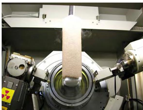
**Figure 2: LN cold-finger sample stage fitted onto an environmental cell on the diffractometer to prevent ice from forming on the sample during analysis. Note the ice forming where the cold-finger sits outside of the cell.**
