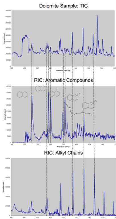
Figure 1. Total Ion Current (TIC) and Reconstructed Ion Current (RIC) Chromatograms of the a Dolomite Sample from Ebbadalen, Svalbard, analyzed on the *Griffin* GC-ITMS using the one-step heating pyrolysis protocol of the SAM instrument to 900 °C.
