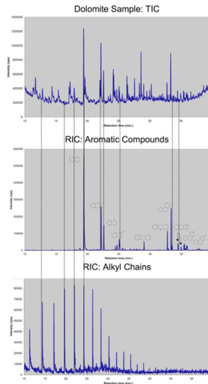
Figure 2. Total Ion Current (TIC) and Reconstructed Ion Current (RIC) Chromatograms of the a Dolomite Sample from Ebbadalen, Svalbard, analyzed on the *Finnigan* GC-QMS using the step-wise heating pyrolysis protocol of the SAM instrument (steps at 300, 450 and 700 °C before heating to 900 °C).
