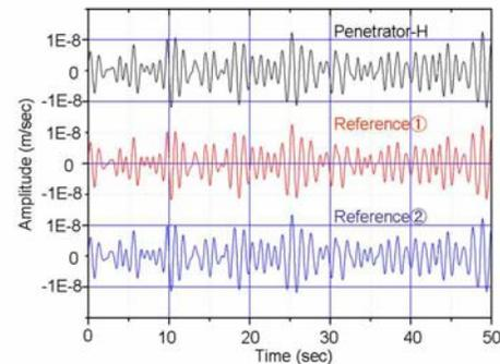
Figure.1 Comparison of waveforms observed by the horizontal seismometers. (Upper line) A waveform by the seismometer on-board the penetrator (Middle line) A waveform by the same type of seismometer without penetrator (Lower line) A waveform by L-4 geophone
