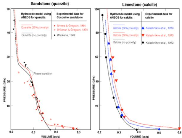
**Fig 1:** Hugoniot curves for different porosities of sandstone (left) and limestone (right).
