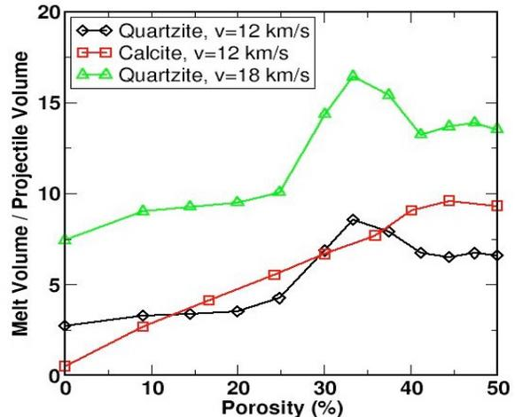
**Fig. 3:** Melt volume relative to projectile volume as a function of porosity for quartzite and calcite.
