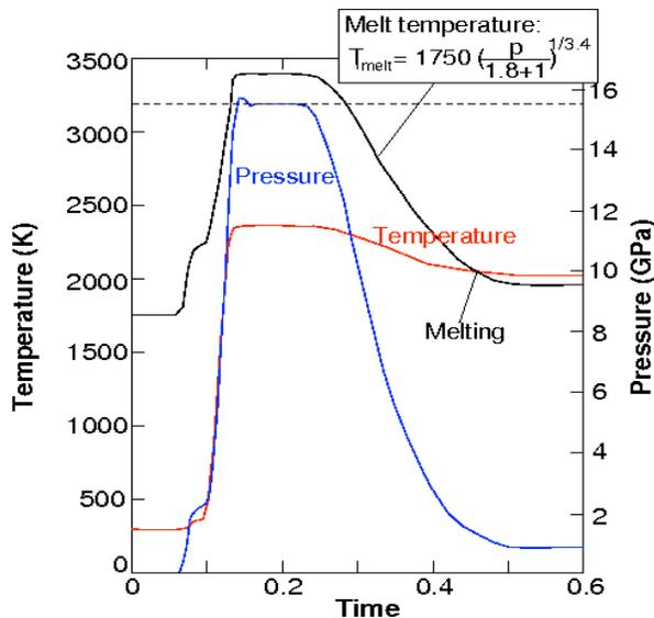
**Fig. 2:** Thermodynamic path (pressure, temperature, and melt-temperature) experienced by a material tracer during the passage of a shock wave. The material is 44% porous quartzite. The parameters for the Simon approximation to calculate melt temperature as function of pressure were taken from [8]
