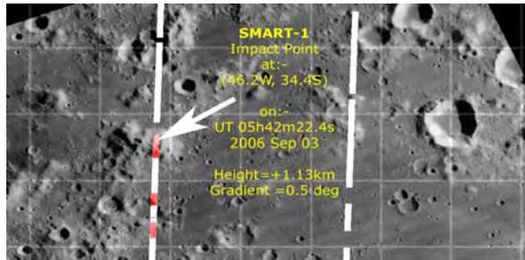
**Fig 3** – The impact site identified on an image taken with AMIE on SMART-1. It corresponds to the location found using the reference craters (see Fig 2).
