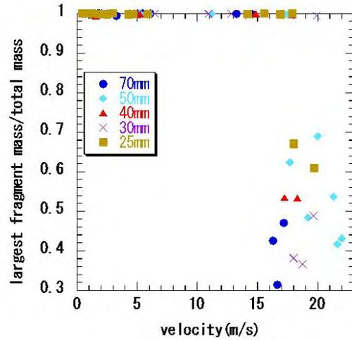
Figure 3: Relationship between the largest fragment mass over the total mass and the impact velocity.
