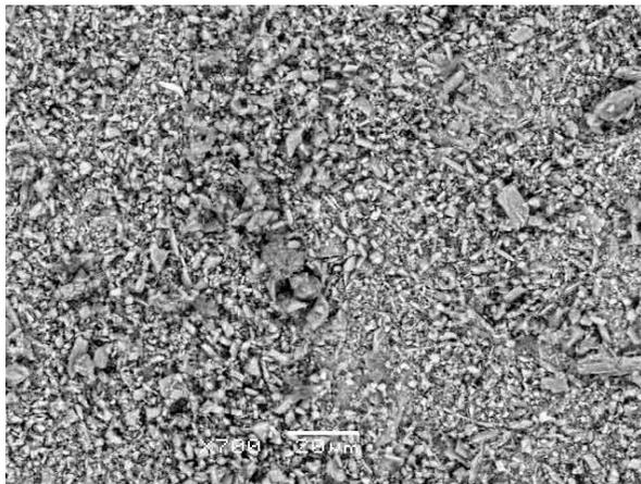
Figure 2: SEM images of a post-impact gypsum sphere. The upper image shows the area near the impact point and the lower image shows the central part of the sphere. The diameter of the sphere was 30mm and the impact velocity was 0.89m/s. The range of scale bars is 20  $\mu$  m.
