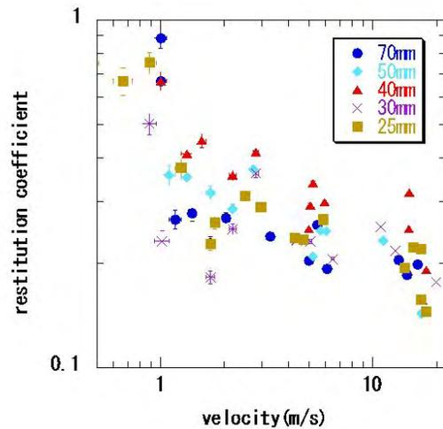
Figure 4: Relationship between the restitution coefficient and the impact velocity. The values became low from about 1m/s.
