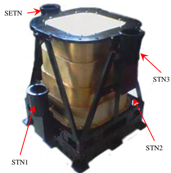
Fig. 1. The Lunar Exploration Neutron Detector. Four sensors of neutrons are shown: 2 open filed sensors of thermal (STN 3) and epithermal neutrons (SETN), 2 sensors of Doppler filter for thermal neutrons (STN 1 and STN 2). Other five sensors are inside the collimator module: 4 collimated sensors (CSETN 1- 4) of epithermal neutrons and 1 collimated sensor of high energy neutrons (SHEN).
