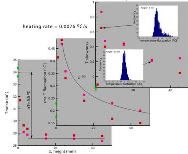
Figure 3. Mean temperature, root mean square temperature fluctuation, and skewness of temperature time series as a function of height above heated bottom boundary.
