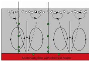
Figure 2. Schematic of experiment. Green symbols show thermocouples. Heater shown in red. White symbols are buoyant particles
