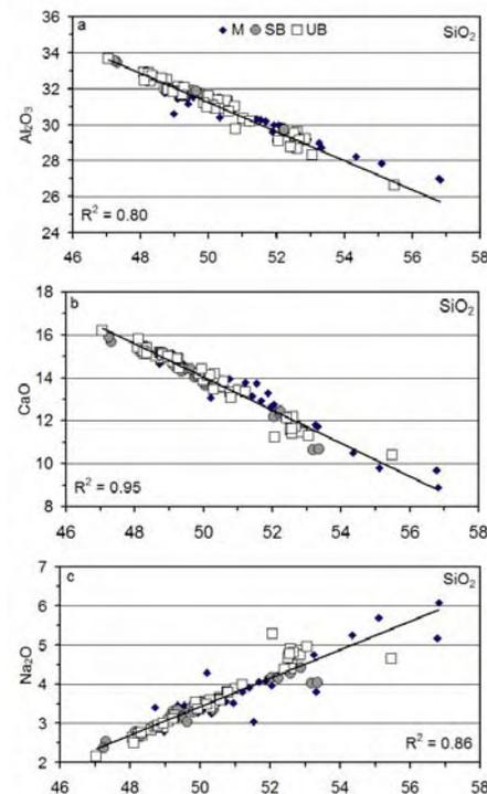
**Fig. 3.** Plots of plagioclase from unshocked basalt (UB), partially shocked basalt (SB), and maskelynite (M) in major oxide bivariate plots.
