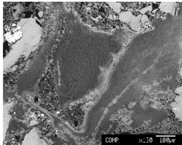
**Fig. 2.** BSE image of maskelynite showing flowage structure, darker gray portion is maskelynite. Sample L60G.
