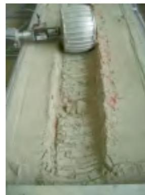
**Figure 3.** MER wheel test in layered soil at the German Aerospace Center (Richter and Schmit).
