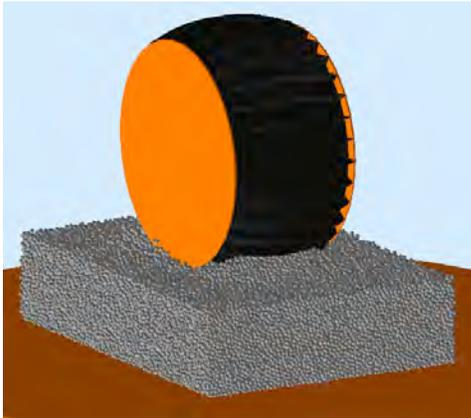
**Figure 4.** DEM 10 simulation of a MER wheel in soil (Hopkins and Kaempfer).
