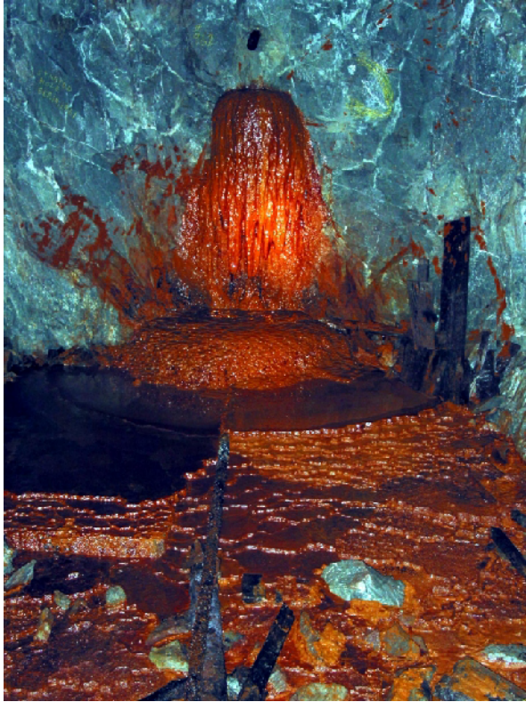
Fig. 2. Diamond drill hole #963. Iron rich deposits on the 27 th level of the Soudan Mine. The view is about 4 m high by 3 m wide.
