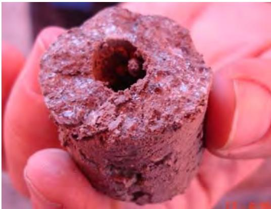
Figure 2. The first core retrieved from a depth of around 45-50cm confirmed the boundary of permafrost layer.
