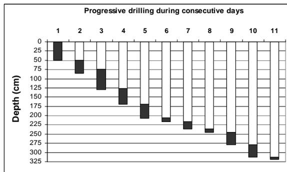
Figure 1. Drilling depth reached during consecutive days. The final depth was 3.19 m, which is new Devon Island record.
