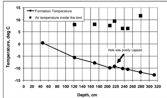
Figure 5. Temperature profile of the permafrost as measured at the bottom of the drilled hole each at the beginning of each field day. Also plotted is the ambient air temperature.
