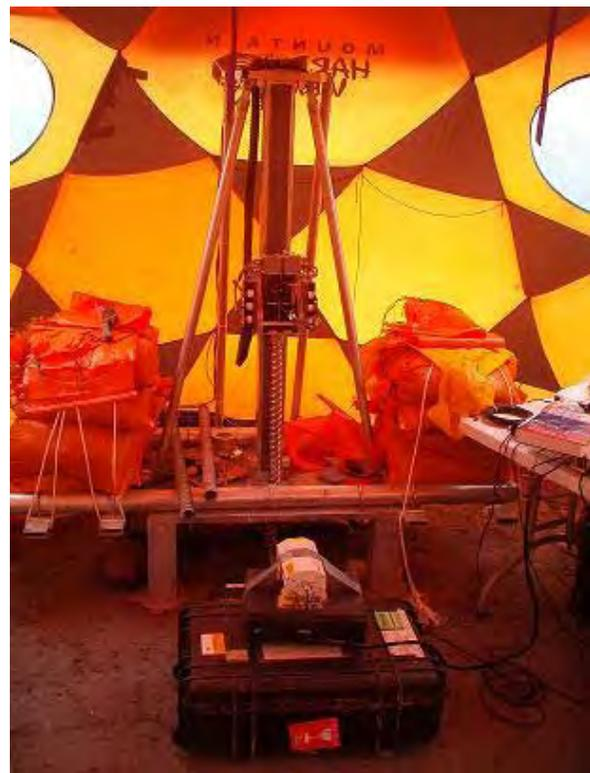
Figure 3. DAME Drill during 2006 field test on Devon Island, Nunavut Canada.
