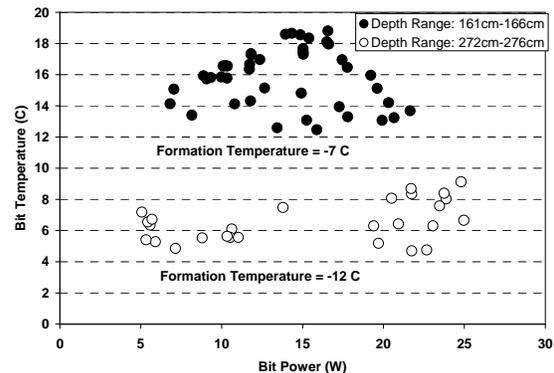
Figure 6. Bit Temperature (°C) vs. Bit Power (Watts) in the depth ranges of 161 cm to 166 cm and 272 cm to 276 cm.
