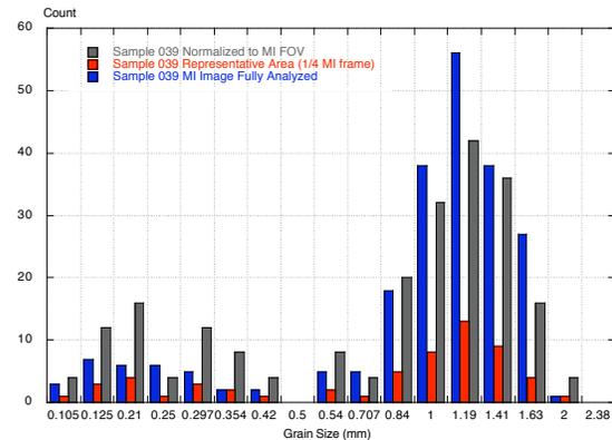
Figure 1: Sol 039 grain-size distribution from: Red - representative area (25% of the entire frame); Grey - results from the representative area normalized to the entire MI Field-of-View (FOV); Blue - count of all measurable particles in the entire frame.
