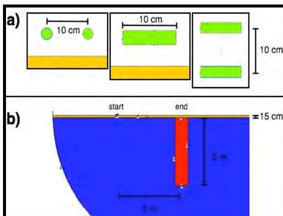
**Figure 1:** Simulation geometry a) shows cross sections of the detector tubes, while b) shows the crack (red) with start and end points of the traverse labeled.
