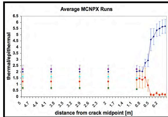
**Figure 2:** MCNPX thermal/epithermal count ratios for several traverses toward an ice-rich and desiccated crack (start position at left). *blue line:* traverse toward a pure water ice filled crack; *red line:* traverse toward a desiccated crack; approaches toward a desiccated crack are shown with 5% (*green points*), 30% (*cyan points*) and 50% (*purple points*) ice in the regolith.
