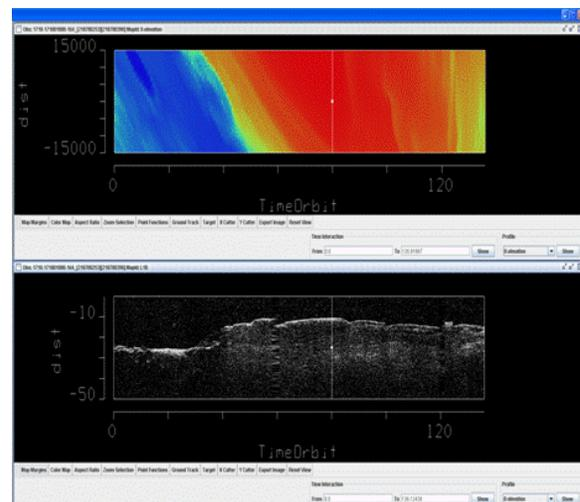
Fig. 4 Graphic Visualization Tool interactive panel showing 2D MOLA scenario compared to the relative radargram.
