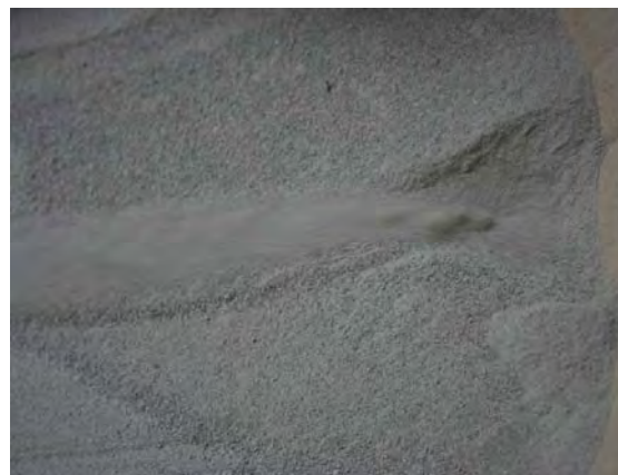
Figure 1. Gully reproduced at laboratory. It can be seen the fluidification effect of the dry sand when air is injected inside the slope. The length of the slope is roughly 20 cm.
