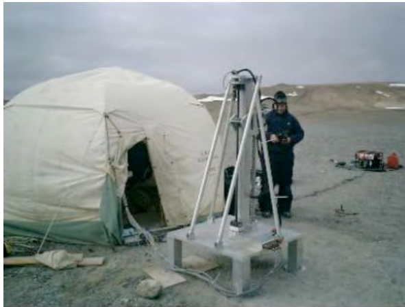
Fig. 1. DAME planetary drill prototype at Devon Island analog test site (Haughton Crater).
