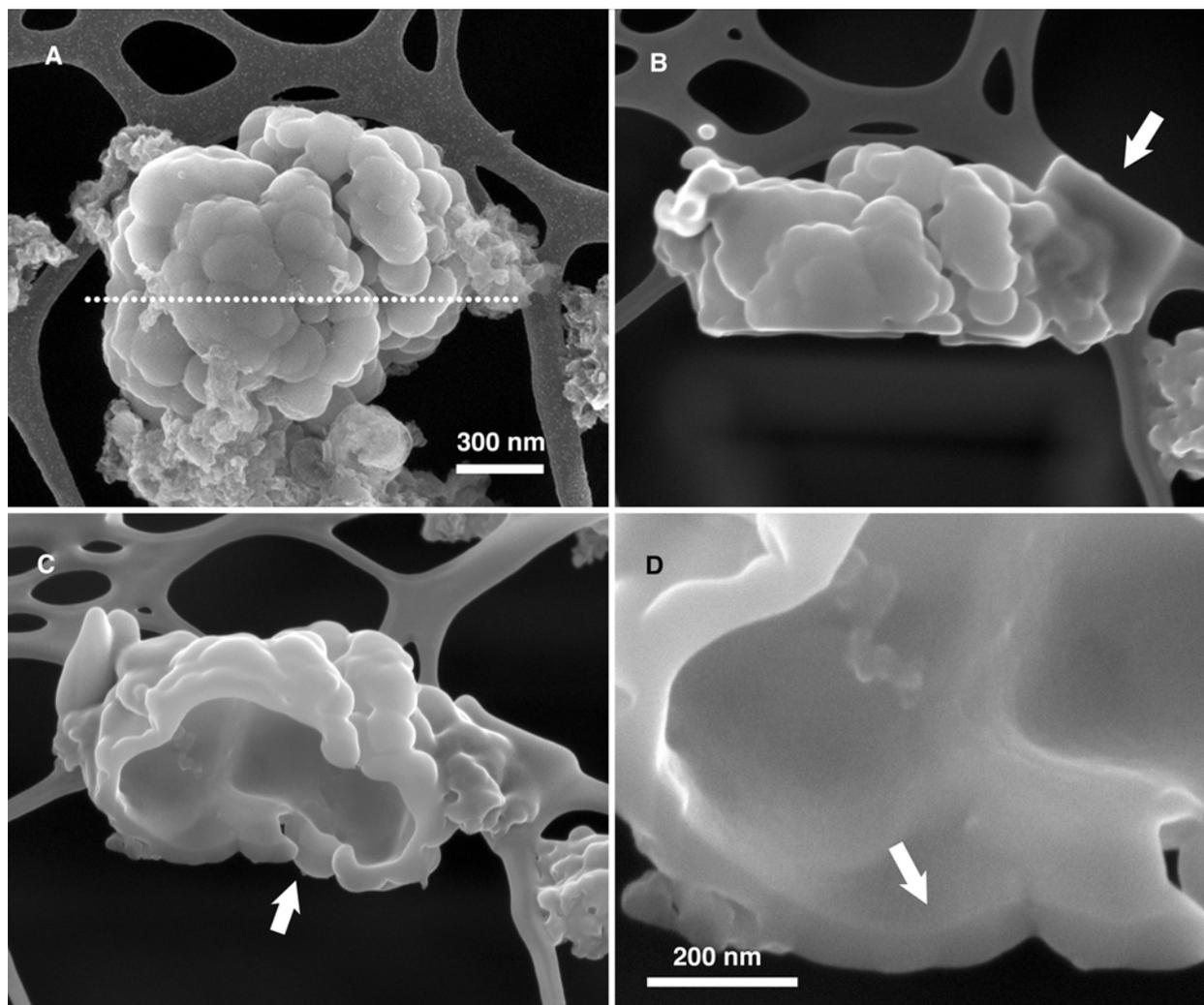
Fig. 1. SEM image (SE mode) of a large nanoglobule supported on a lacey C TEM grid (A). The dotted line shows where the globule was sectioned. B) Milled globule. Arrowed square area shows where Pt was deposited between the globule and the supporting film to prevent the particle falling away from the TEM grid during milling. C) Particle tilted 25° showing the hollow interior. The arrow points to an opening in the globule wall. D) Close up showing the details of the interior and globule wall.
