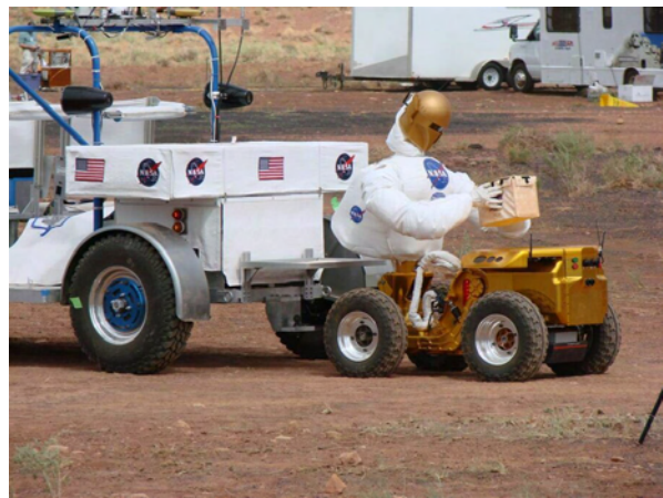
Figure 3: Centaur autonomously removes and stows a sample box
