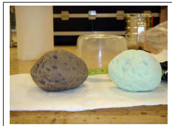
Figure 3 Image of the field sample of vesicular basalt cobble (left) and the printed model of target (right).
