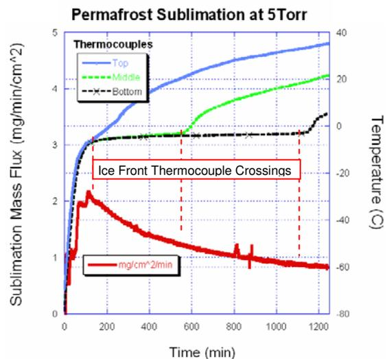
**Figure 4.** Experiment for determining sublimation rate as a function of ice table temperature.
