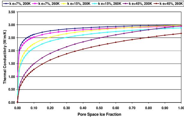
**Figure 2.** Icy Regolith Thermal Conductivity vs. Pore Space Ice Fraction for porosity = 7%, 15%, 45% and Ice Temperatures of 200K and 260K.
