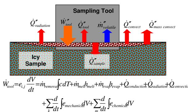
**Fig 1.** Power balance of sampling tool heat and mass transfer interactions with an icy sample.
