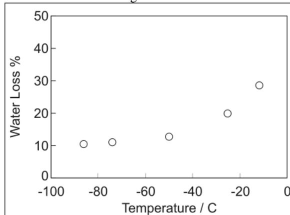
**Figure 5.** Water loss percentage vs. temperature for saturated (~23% water wt/wt) permafrost pucks.
