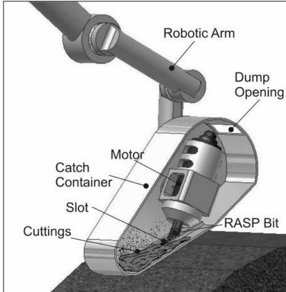
**Figure 1.** Diagram showing RASP on a robotic arm with collected sample.
