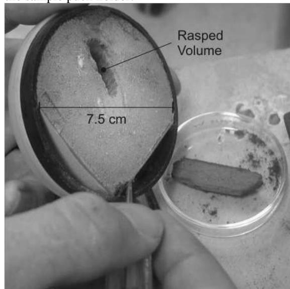
**Figure 4.** Sample puck showing Rased hole and the portion of the sample used to measure water content in the Petri in the lower right.
