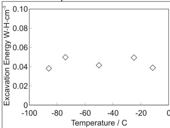
**Figure 2.** RASP excavation energy per unit volume.
