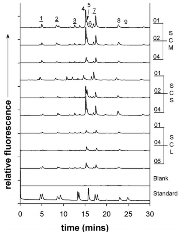
**Figure 2.** HPLC chromatograms of total hydrolyzable amino acids (THAA) detected in small (SCS), medium (SCM), and large (SCL) Sunset Cliffs ironstone concretions. 1=D/L-aspartic acid, 2=L/D-glutamic acid, 3=D/L-serine, 4=glycine, 5= $\beta$ -alanine, 6= $\gamma$ -aminobutyric acid, 7=D/L-alanine, 8=L-valine, 9=D-valine.
