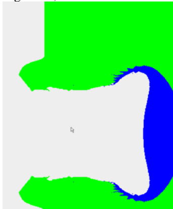
Figure1 shows simulation example when iron impacts porous quartz (400x300 cells, 2D). At this some cells contain two materials at the same time. The iron meteorite still moves toward while the target material blows outwards.
