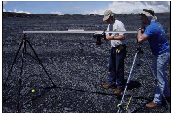
Figure 1. Example field set-up. 12.8 megapixel camera is suspended between two tripods. Images are taken every 10 cm and stereo matching is performed back in the lab.
