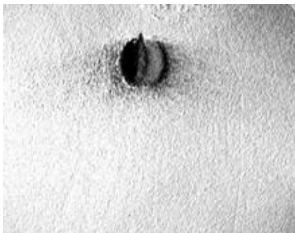
Figure 6. 0.5^\circ Impact. Crater is 49 mm x 42 mm. Ejecta is concentrated in the crossrange direction, with some ejecta still present in the downrange direction. Projectile trajectory is from top to bottom.
