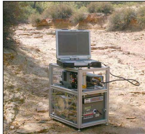
**Figure 1. CheMin 4 instrument in Rio Tinto river bed with optional laptop computer for graphic user interface.**
