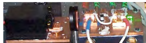
Figure 5: Ten inch prototype of Yb:YAG development for laser ablation; diode on left (black box) & 2 amplifiers on right; smaller package to be delivered in 2007.
