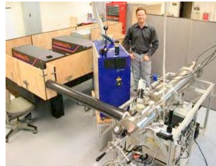
Figure 3: Lab version of LARIMS complete, ready to define requirements for miniature system.
