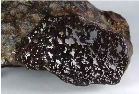
Figure 1: Cut face (3.3 cm wide) of NWA 2993 showing 30 vol.% fresh metal and coarse mafic silicates.
