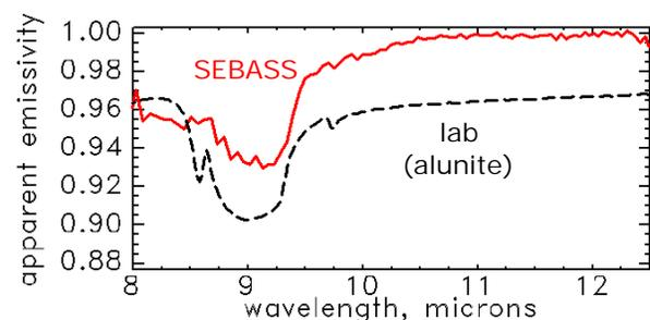
**Fig. 2:** SEBASS vs. lab spectrum. Laboratory sample is ASTER so04ac ( $150\text{--}500\ \mu\text{m}$  particles), scaled to plot with similar spectral contrast as SEBASS for comparison of the band shapes. SEBASS is pixel x1181/y26, shot 060501\_165938\_aln2.
