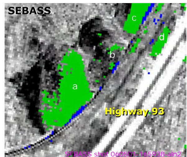
**Fig. 7:** SEBASS mapping of alunite (green) and gypsum (blue) signatures. Signatures mapped are from the ASTER on-line library, of alunite sample “so04ac” and gypsum sample “so02bc”, both particle size 125 to 500  $\mu\text{m}$ . Gray image is the 9.44  $\mu\text{m}$  SEBASS band.
