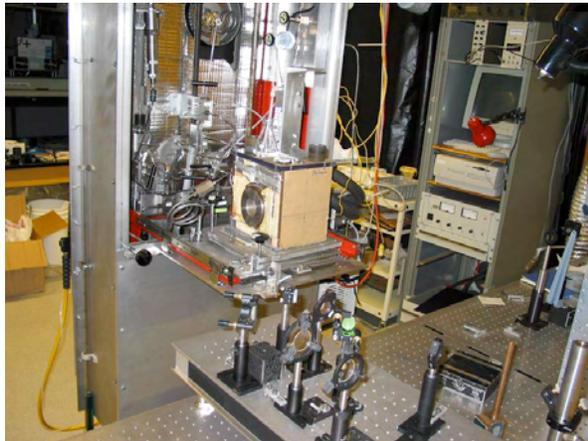
**Figure 1.** Front view of the icy satellite interior simulator. The cylindrical pressure vessel is shown, contained in an insulating box. In front of ISIS is the setup for impulsive stimulated scattering, which can be used to measure sound velocities and thermal diffusivities [8,9,10].
