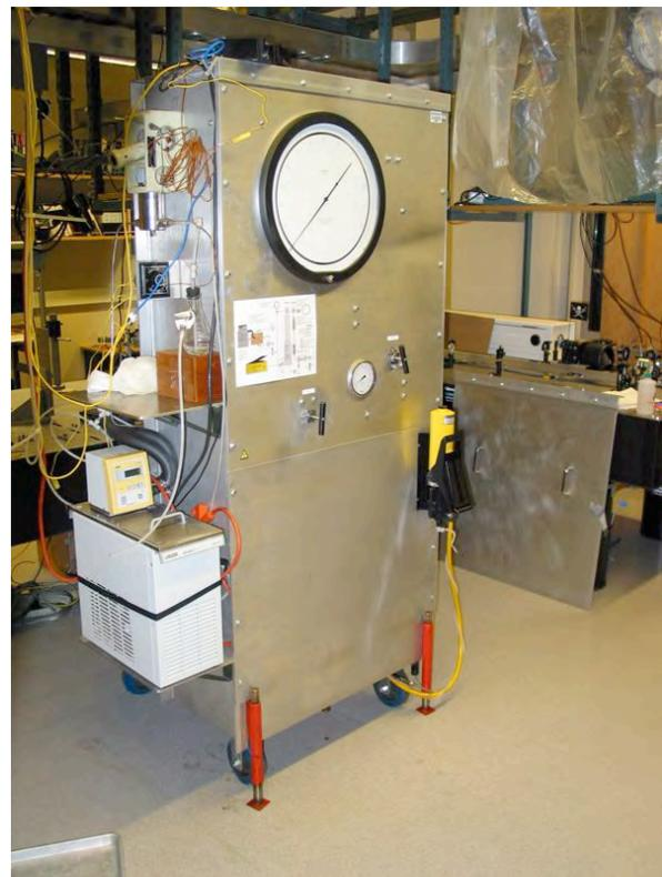
**Figure 2.** The icy satellite interior simulator, rear view. The Lauda circulating heater/chiller is shown the left. The air-driven hydraulic pump is attached on the right.
