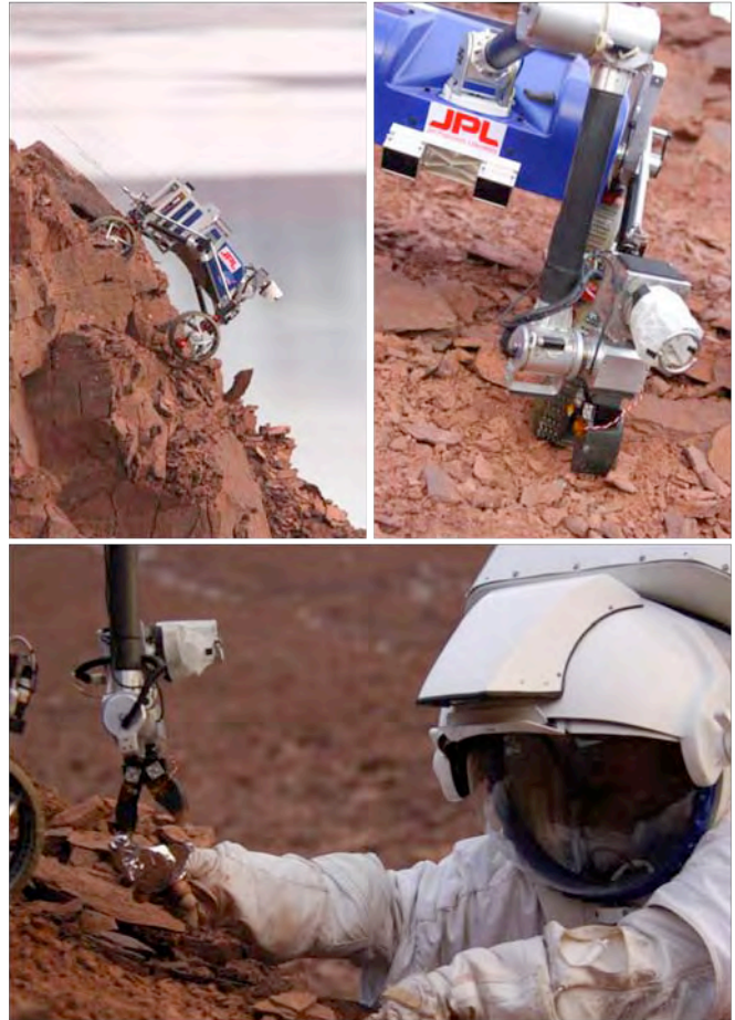
Figure 1. Field deployment of the JPL TRESSA system on Devonian Red Beds at the BVC site. A) shows the steepness of the slope on which the rover is operating. B) shows the rover taking a sample with its integrated scoop. C) shows the rover handing off the sample to the Mark III space suit astronaut.
