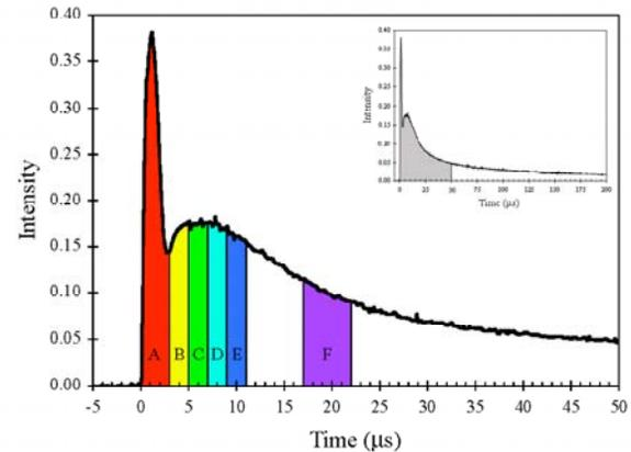
**Figure 1.** The location of the six short-exposure camera images (A-F) with respect to the photodiode light curve. The light curve out to 200  $\mu$ s is shown for context, with the shaded region corresponding to the duration depicted in the main graph.
