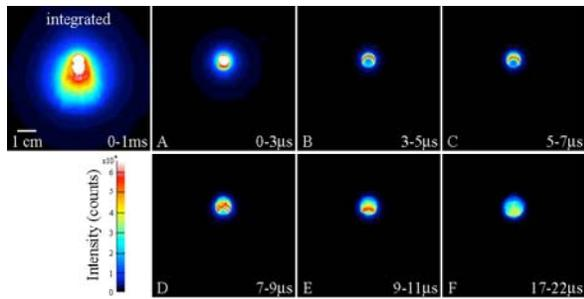
**Figure 2.** A composite time series representing the impact flash intensity for a Pyrex projectile impact into pumice dust at 60°, with a velocity between 1.6 and 1.9 km/s. The first image is an integrated image of the entire impact flash. The subsequent images (A-F) are much shorter exposures, as noted.
