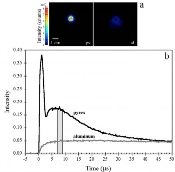
**Figure 3.** Comparison of Pyrex and aluminum projectiles. (a) Two  $\mu\text{s}$  exposures of Pyrex (px) and aluminum (al) impacts taken 7 and 8  $\mu\text{s}$  after impact, respectively. (b) Comparison of the two light curves. The approximate time of exposure is shaded.
