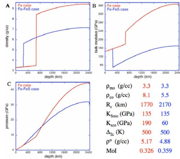
**Fig. 2** - Density (A), bulk modulus (B), and pressure (C) as a function of depth for our two end-member models. The red model has a pure solid iron core [16] and the blue model has a liquid Fe-FeS core (10 wt% S) [19]. Both models have the same mantle and thermal parameters. The low pressure, low temperature input parameters and resulting decompressed density and moment of inertia for each model are shown.
