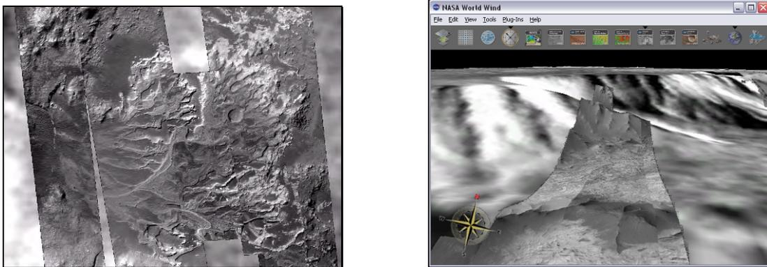
**Figure 1.** The left image shows an example area of the MOC NA mosaic streamed live from the OnMars JPL WMS server (23.8S, 326.4E, 31km across). The image on the right shows NASA's World Wind, a 3D application, displaying the live MOC NA mosaic over the much lower resolution MDIM21, both layers draped in 3D over the MOLA DEM (4.8S, 282.85E, 1X). URL: <http://worldwind.arc.nasa.gov/>.
