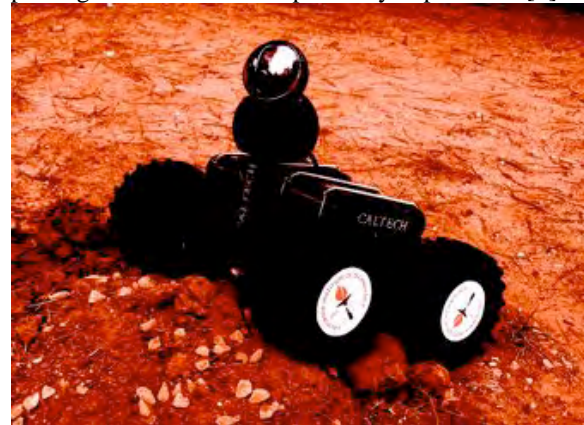
Fig. 2. 4WD remote controllable robotic platform as a representative mobile ground-tier agent of the tier-scalable reconnaissance mission test bed.
