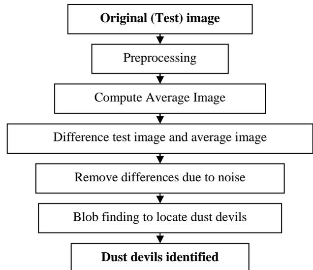
**Figure 2.** Dust devil detection algorithm.
