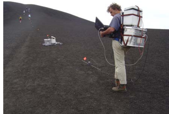
Fig. 1. The positioning layout of a GPR survey conducted over the tephra-covered Inferno Cone at Craters of the Moon National Monument.
