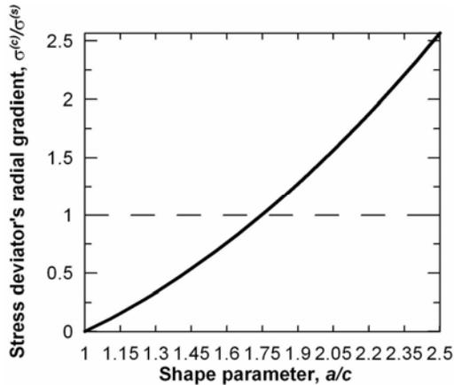
**Fig. 2.** Dependence of a radial gradient of the stress deviator on shape parameters.  $\sigma^{(c)}$  - stress deviator in the center;  $\sigma^{(s)}$  - stress deviator on the surface;  $a > c$  - semi axes.
