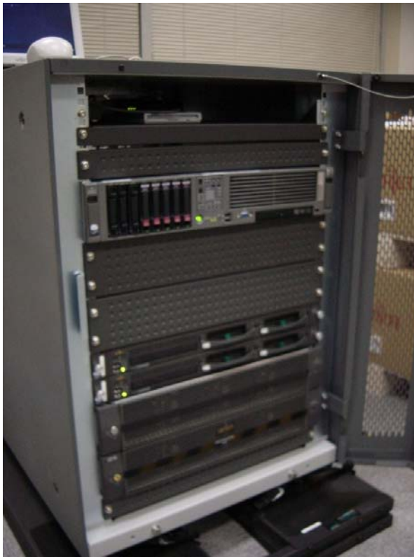
Fig. 2. The photograph of the Kaguya science data WebGIS system. The lowermost machine is the storage, and middle two machines are web server and database server. Uppermost server is WMS/DB server.
